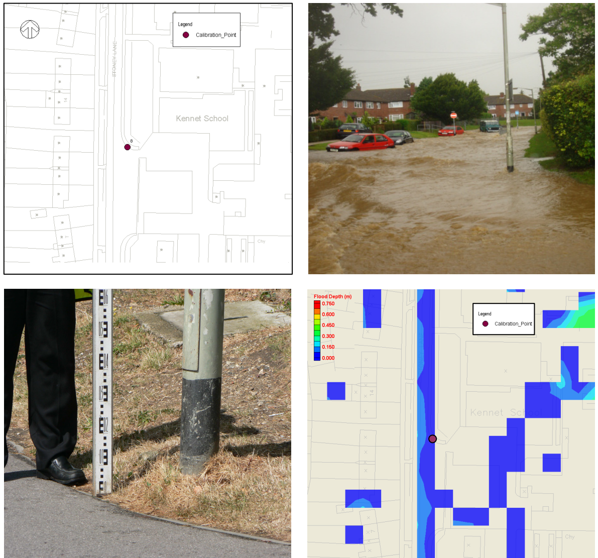
Figure 3-2 Location of model verification point, photograph of flooding in 2007, photograph of on-site measurements and modelled output
