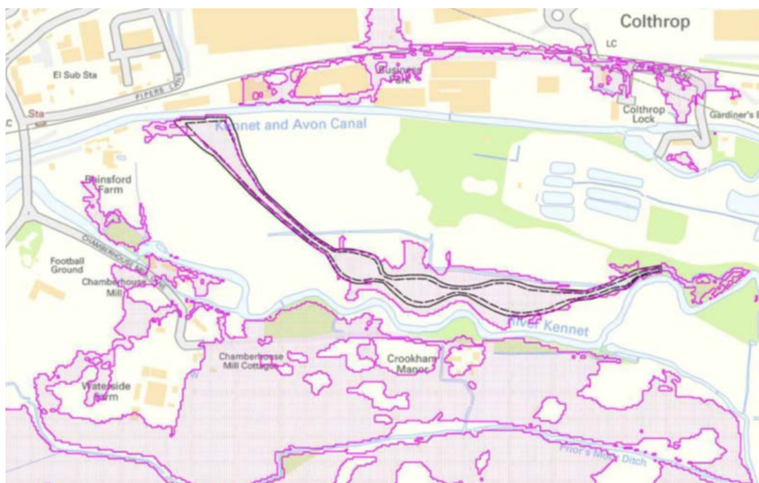
Figure 16: Proposed fluvial flood mitigation strategy with modified 1 in 100 flooding event area
