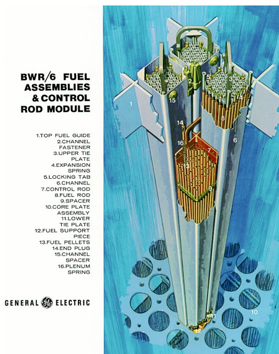
Figure 4: Boiling Water Reactor Fuel Assemblies and Control Rod Module (figure courtesy of GE Hitachi Nuclear Energy)
