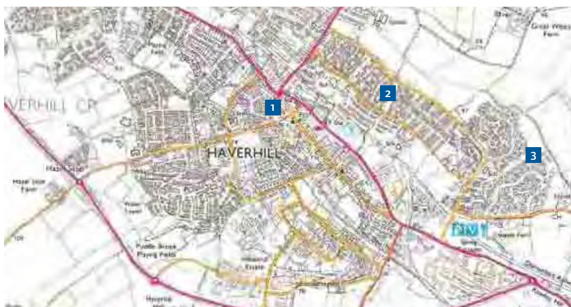
Figure 4.5 The plans of many UK villages, towns and cities illustrate different patterns of development over time, from (1) historic cores, through to (2) experimental 'Radburn' layouts from the 1960s, to (3) recent cul-de-sac/DB32-type layouts.
