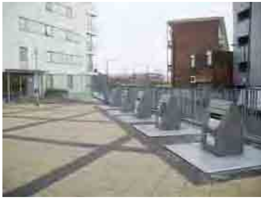
Figure 5.10 Sub-surface recycling bins for communal use.
