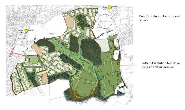
C) The orientation and slopes issues based on plans from WBC site.
