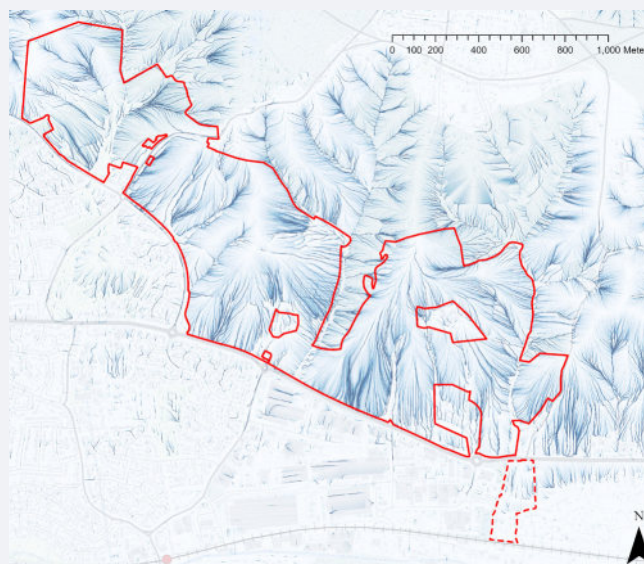
Figure 52: Flow accumulation map showing drainage path concentrations
