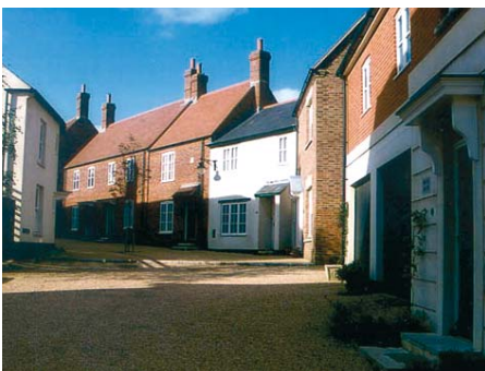
Front to front distances can be reduced to 9m as long as each dwelling is carefully designed
