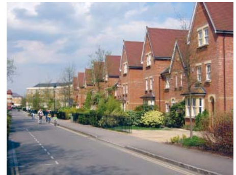
Set back from the footway provides room for a small garden and parking area
