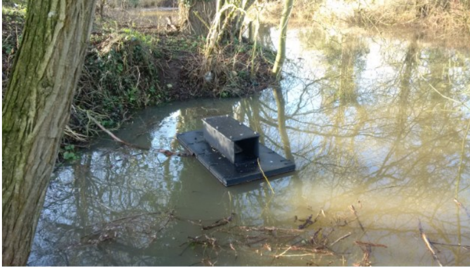
Float containing clay filled basket to detect footprints
